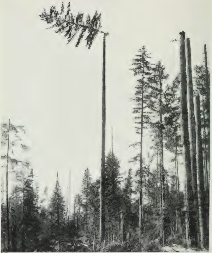
FIG 49. TOPPING SPAR TREE FOR HIGH LEAD: BRITISH COLUMBIA. [By courtesy of British Columbia Government.]
